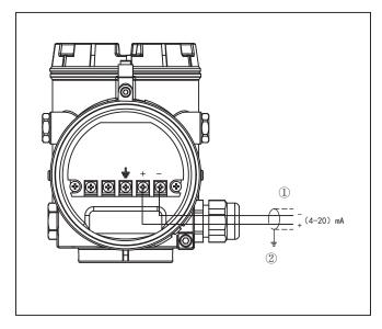
Electronics and terminal compartment, double chamber housing
